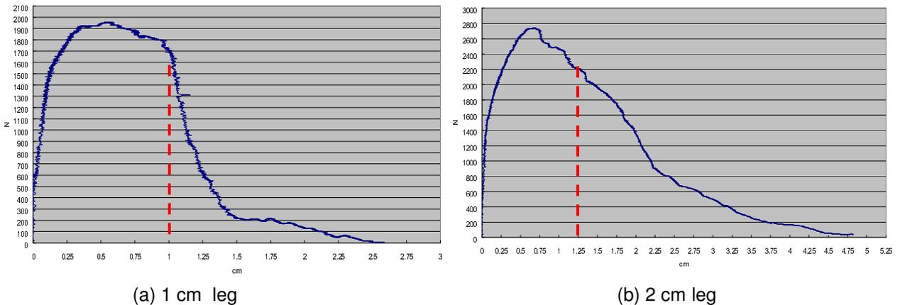
Figure 6. Force-Displacement curve of B&Q on wood.
