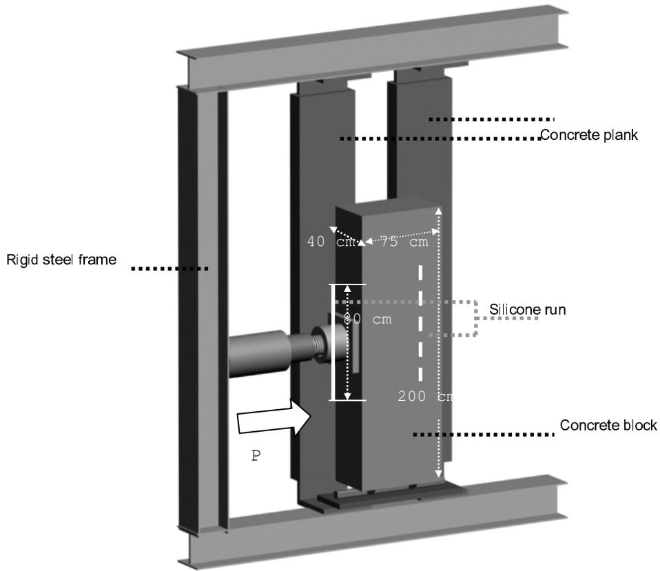
Figure 4. Test set-up of the silicone strength.
