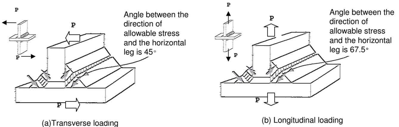
Figure 2. Different loading directions with respect to the weld.
