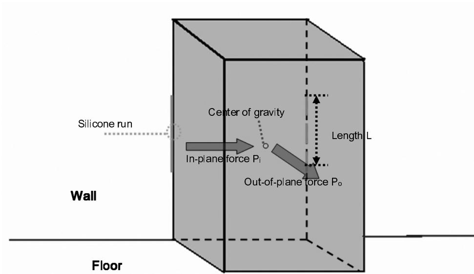
Figure 3. Schematic drawing of a cabinet adhered to the back wall under earthquake excitation.
