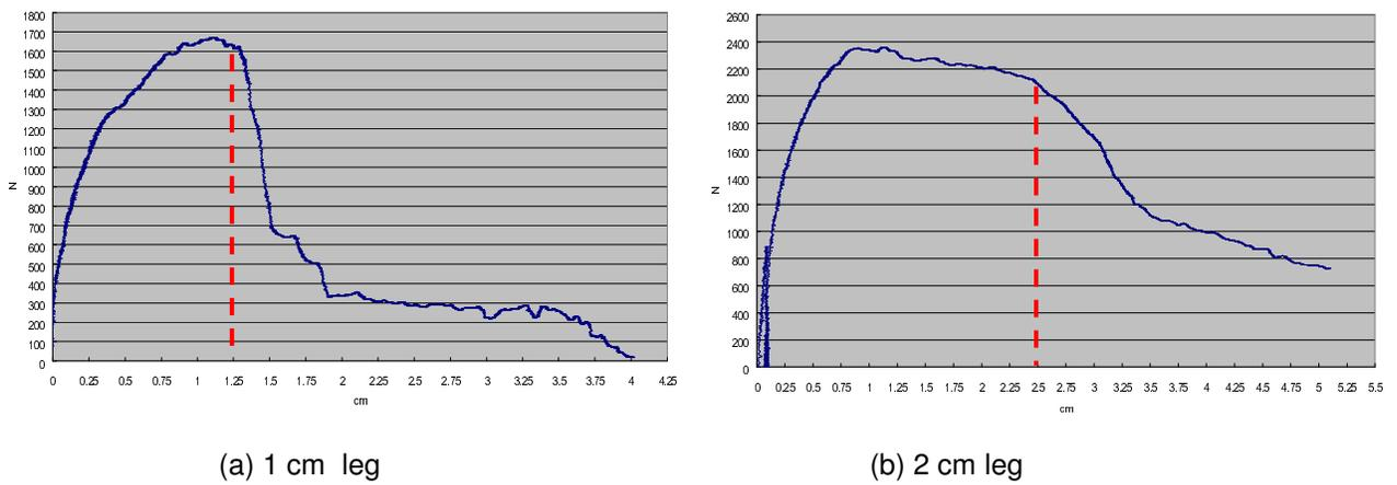
Figure 5. Force-Displacement curve of DC-795 on wood.
